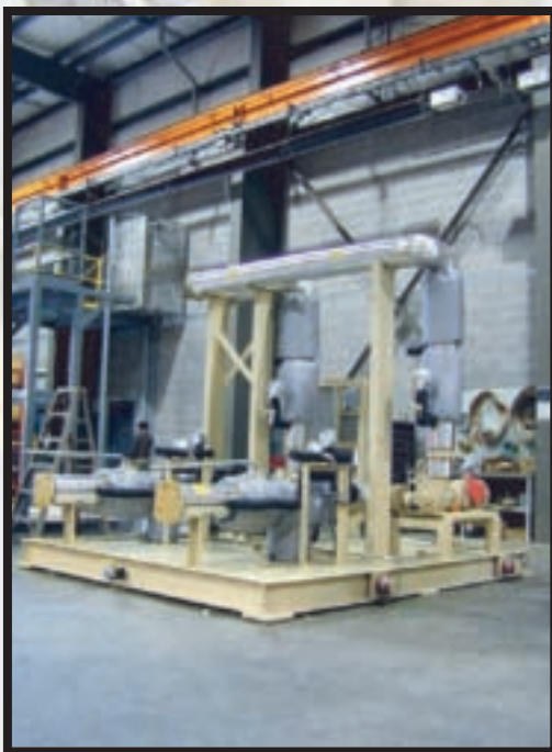
Liquid Process Unloading System
