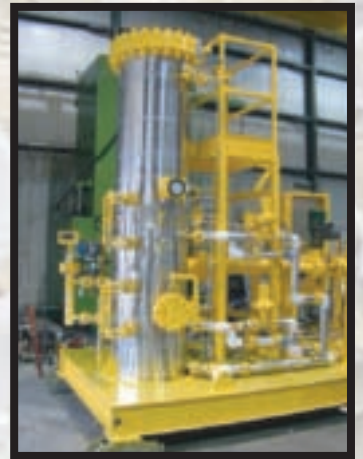
Detail: Coalescer Filter Vessel
